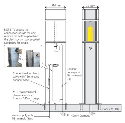
Install detail for the Aquafil Water Refill Station with internal drainage For freestanding mounting to concrete slab close to a building wall with rear entry for water and drainage feed
