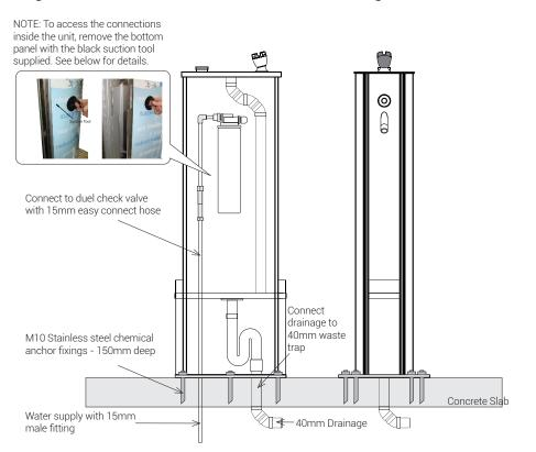
For freestanding mounting to concrete slab close to a building wall with rear entry for water and drainage feed
