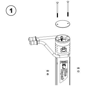
Remove the 3/8" nut and penta tamper-proof nut from the underside of the top cmpartment and lift out the carriage bolts. These are all best removed with a socket wrench, using the extension tool to enable you to reach the nuts.
