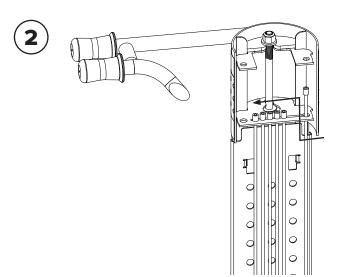
Add or remove tools by sliding the tool cables through the hole at the end of the cable slot in the Fixit Plus upright.
