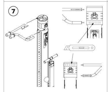
Select the orientation of the bike hanger and use a new razor blade to cut through the decal to reveal the corresponding slot in the Fixit Plus.
