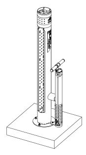
Place the Fixit Plus over the anchors, add washers and nuts, and tighten all nuts.
