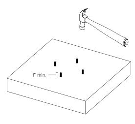
Hammer in the (4) 3/8" wedge anchors. Leave at least 1" inch of exposed threads above the concrete.
