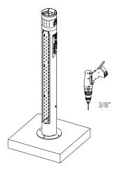
Reference the Fixit Plus setback recommendations and place the upright in the desired location. Use the base as a template to mark anchor locations and drill (4)  $3/8" \times 3"$  holes in the concrete with a hammer drill and masonry bit. Clean up all concrete dust from drilling.
