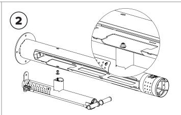
Secure the Air Kit to the side of the Fixit Plus with the 3/8" threaded stud on the Air Kit and a bonded washer and lock nut inside the Fixit Plus.
