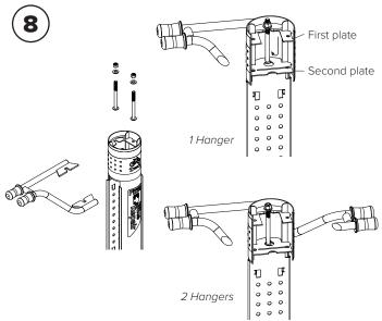
Add the 1/2" washer and 1/2" lock nut to the 1/2" x 6" carriage bolt. Insert the assembled hardware, headfirst, into the top of the Fixit Plus. The carriage bolt head will pass through the second plate hole and then slide sideways, so the carriage bolt engages the slot in both plates and bike hanger. Tighten the lock nut and repeat with the other side. If two bike hangers are used, the carriage bolt will also engage the second bike hanger under the second plate.
